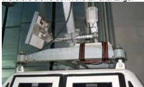
Figure 1: Air temperature, humidity and pressure measurement on a Gondola at the Planai ski resort (Schladming, Austria).
